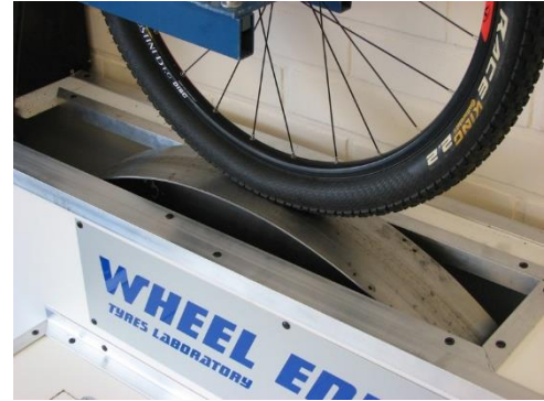
Fig. 2. Rolling Resistance testing machine at Wheel Energy.
