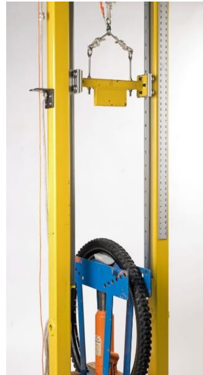
Fig. 5. Measuring impact force dissipation on our drop test tower.
